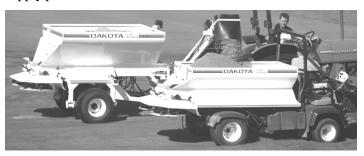
There are two positions for the side conveyor. The **traveling position** is when the side conveyor is retracted and rests against the side of the hopper. The **operating position** is when the side conveyor is fully extended to the side.
