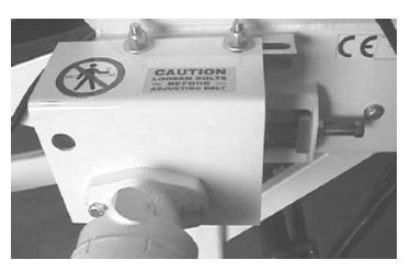
3. Using a ¾ inch wrench, turn each tensioning bolt clockwise 1-2 complete turns. Be sure to make equal adjustments on both sides.
