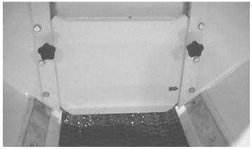
The rear metering gate is designed to regulate the flow of material out of the hopper. Two types of the metering gate are available: hand crank, or manual opening.
