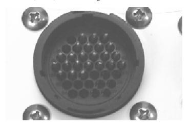
If after uncoupling the Turf Tender on trailer-type models, it has happened that the operator drove off without disconnecting the power cable from the tractor and forgetting to return the control box to its storage location the connector may get damaged.
