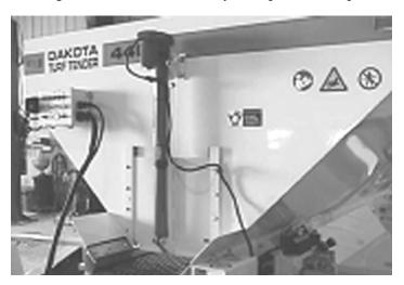
The electric front gate is easy to operate. One switch moves the gate either up or down. Push the switch away from the tractor operator and hold to open the gate. Pull the switch toward the operator and hold to close the gate. Releasing the switch will stop the gate at whatever position it is in.
