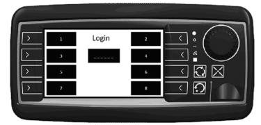
The Login screen will show when the Login button is pressed from the Menu screen. The Login screen is to be used to access either the OEM Setup or the Calibration screens. Entering the appropriate password will access the desired screen. If the password is entered incorrectly, the Login page will reset.
