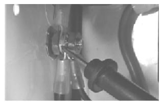
5. Check the voltage between the control box's chassis ground screw (on the left side wall) and the brass buss bar running across the top of the fuse block. If there is no voltage detected, check all connections.
