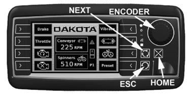
Prior to operation of the Turf Tender, it is highly recommended that the operator go through each of the functions on all screens to become thoroughly familiar with each function and the screen from which it is activated. Practice accessing each function until totally familiar with its function and screen location.
