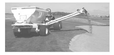
Lowering the side conveyor to its lowest position makes it easier and more accurate for filling trenches, pots, or areas that require some degree of unloading accuracy. With the hood at the end of the conveyor in the down position it forms a spout that helps keep the unloading materials in more of a controlled space and results in less time spent cleaning up.
