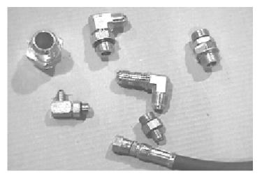
All components use either an O-ring boss or  $37^{\circ}$  flare hydraulic fittings. Do not use pipe-threaded hoses or fittings for replacements. Do not use Teflon tape or pipe thread compound. These are not helpful and may cause damage to the system.
