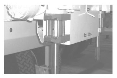
Periodically check the hydraulic hoses for worn areas and other unsafe conditions (cracks or leaks). This should be part of the safety walk around each time before using the Turf Tender. Pinhole leaks under pressure can pierce skin and inject hydraulic oil under your skin. Never handle hoses while the hydraulic system is pressurized.
