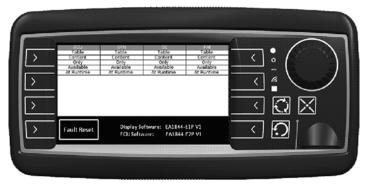
When a fault has been indicated by the fault icon, press the fault button to bring up the fault code table to identify which function is experiencing a fault. Troubleshoot the wiring to the function according to the fault code table. When the fault has been corrected (usually a broken wire, loose connection, or wire grounding on the frame), then press the Fault Reset button to reset the fault.
