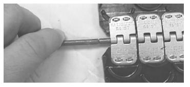
10. Fully insert the new hinge pin into the splice. Use the hinge pin to push the steel rod out of the splice.
