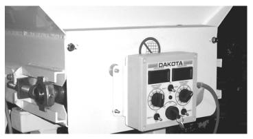
Slide the control box into the mounting bracket on the tractor. Secure by tightening the screws on the back of the bracket.
