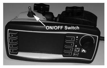
Upon completion of the loading screen, the home screen will be displayed and the controller is now functional. The following hard and soft keys are operational on the home screen. Also, the following will be displayed on the home screen.
