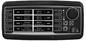
The Calibration screen is used to change the machine calibration settings. When a button is pressed, the Encoder knob will be linked to the corresponding setting and the icon will change in color. The following variables can be adjusted:
